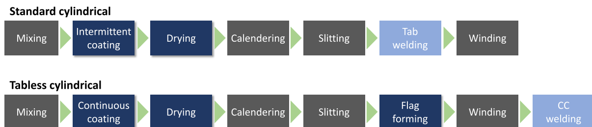
Fig. 5. The manufacturing process steps of creating standard and tabless jellyrolls based on [29]. Process steps that need to be considered to evaluate the cost effects are highlighted in dark blue. (For interpretation of the references to colour in this figure legend, the reader is referred to the web version of this article.)
